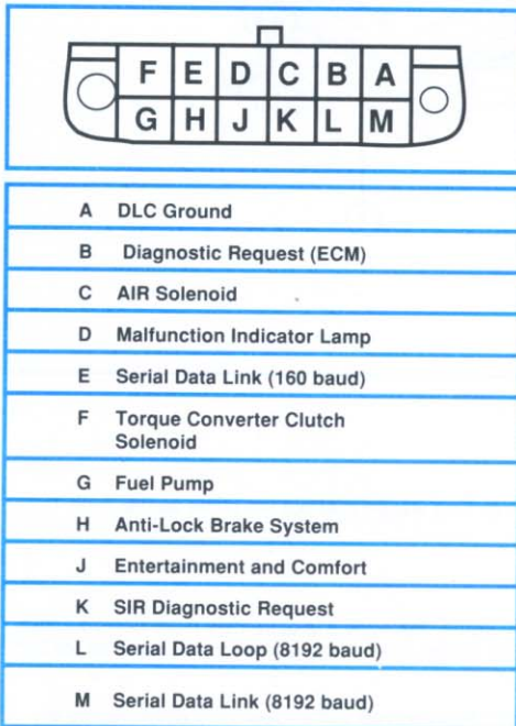
Figure 1-5, DLC (12 PIN) Identification (Typical)
