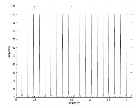
This frequency response tells us our output has a fundamental frequency of 200 Hz with multiples of 200 Hz being our harmonics.
