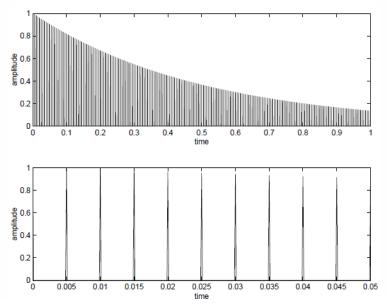
This has a period of 0.005 seconds and a frequency of 200 Hz.
