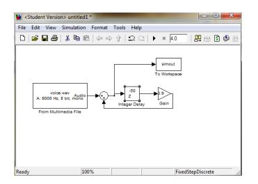
So we have a gain of 0.9 and an N value of 50. If we use a N value of 2000, it tends to echo. If we use N = 50 it's kind of a changed, kind of amplified sound, it is reflecting the sound. The delay bounces around some energy is lost each time it does this. When alpha is greater than 1 it is an unstable system. When alpha is 0, the sound sounds the same as it is the same. When alpha = 1 the sounds echoes forever.
